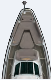
Optional U-sofa Package with removable table and storage underneath, backrest cushions, anchor locker cushions with cupholders, sunbed infill, and Mediterrana Edition.
